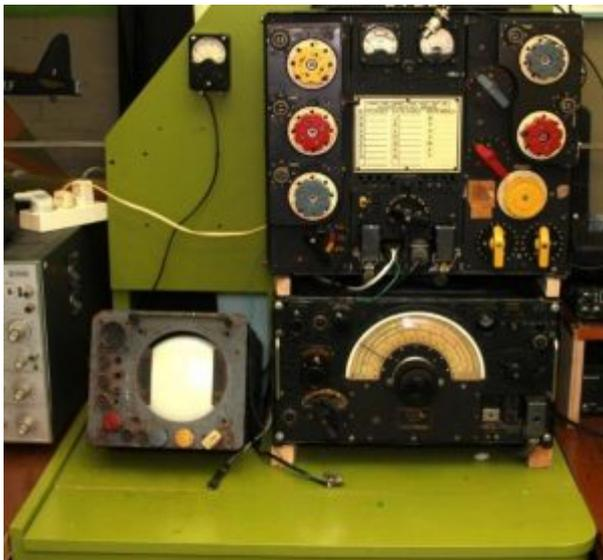
The centrepiece of the radio room is this WW2 RAF Wireless Operators table, complete with R1155 receiver (bottom) and T1154 Transmitter, (top) and a Fishpond indicator (left hand side). This equipment was used in the latter part of the war for long distance morse-code communications between Bomber Command Group Headquarters and aircraft in the air. Underneath are the original ground power supplies.
